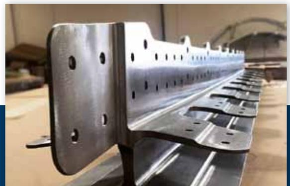
Typical parts produced with Hot Stretch Forming:
