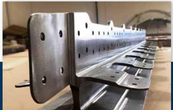
Typical parts produced with Hot Stretch Forming:
