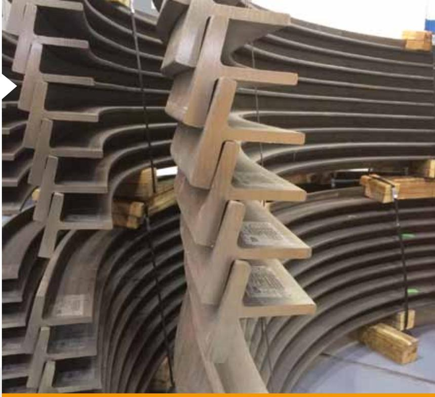
Aries Manufacturing has developed a very innovative Hot Stretch Forming process to contour titanium profiles for airframe component applications. The HSF® process saves material and machining time, which are two serious cost issues for today's aircraft manufacturers. In addition, the process allows for consistent quality in a productively efficient manner, assuring the sustainable attainment of delivery and build schedules.
