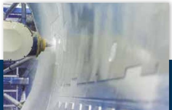
Typical parts produced with MMS®: fuselage aluminum 3D skins to perform pocketing, drilling & routing in a single setup.
